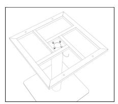
Step 4 Set base end down on the floor on a soft surface to avoid damage to the top. Place the canopy on top with the indented screw plate facing up. Make sure the flat edge of the base aligns with the flat side of the bar (if the bar is square). Align screws and screw in 4 of them about half way. Tighten screws with allan key once all screws are in place.
