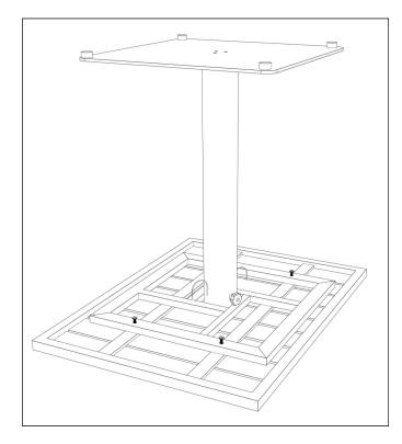
Our umbrella tables have two different types of connectors on the bottom. The 32 x 32 and smaller tables have 3 screws to connect with a square base plate. The 32x48 (and potentially larger) tables connect with 4 screws to a rectangular base plate. The rest of the pole is exactly the same.
