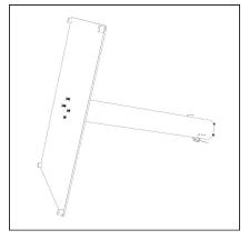
**Step 3A** For the 32x48 Table - Tilt the base against your body and hold the pole against the top of the plate (opposite the feet). Align screws and screw in 4 of them about half way. Make sure the flat side of the base aligns with the flat edge of the bar (if the bar is square). Tighten screws with allan key once all screws are in place.
